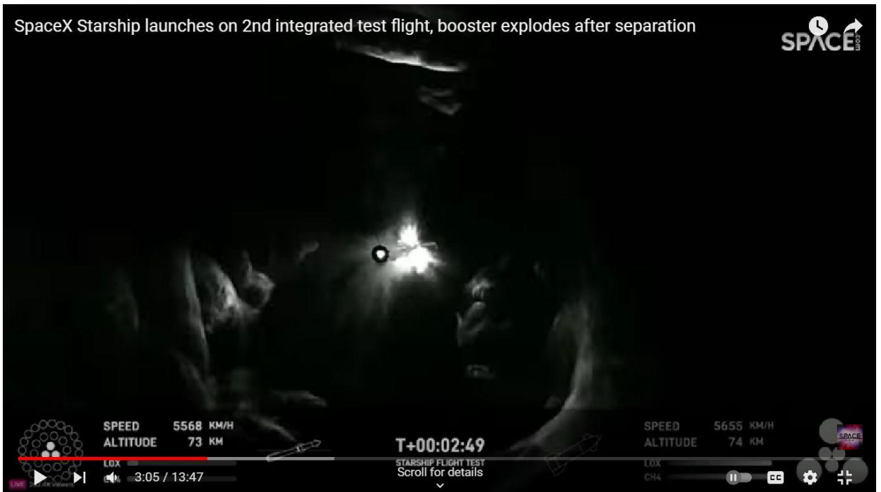
Fig. 2 – The moment of stage separation, the longitudinal axis of the booster approximately coincides with the direction of system flight
