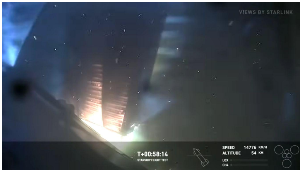
Fig. 7 – Picture of hypersonic flow around the junction of hull with forward flap in the middle of braking
