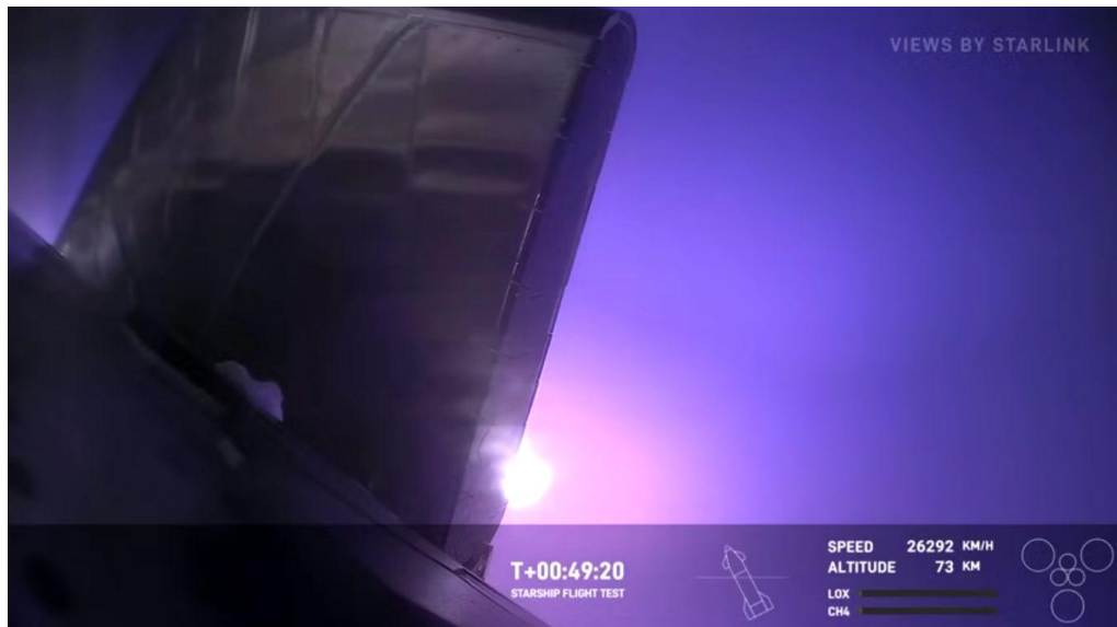
Fig. 6 – Picture of hypersonic flow around the junction of hull with forward flap at the beginning of braking in the atmosphere
