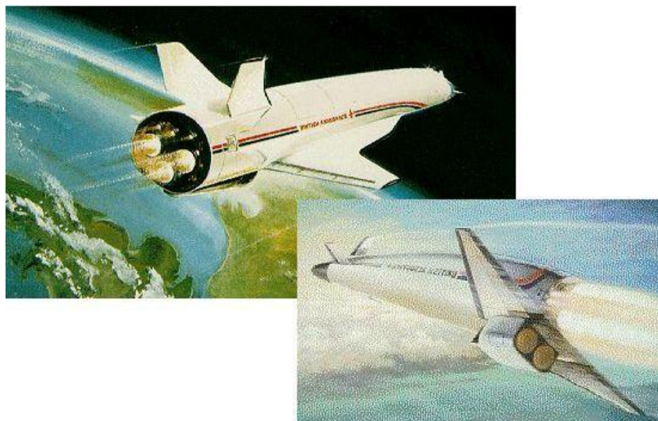
Fig. 9 – Initial (bottom) and final (top) layouts of Hotol orbital aircraft
