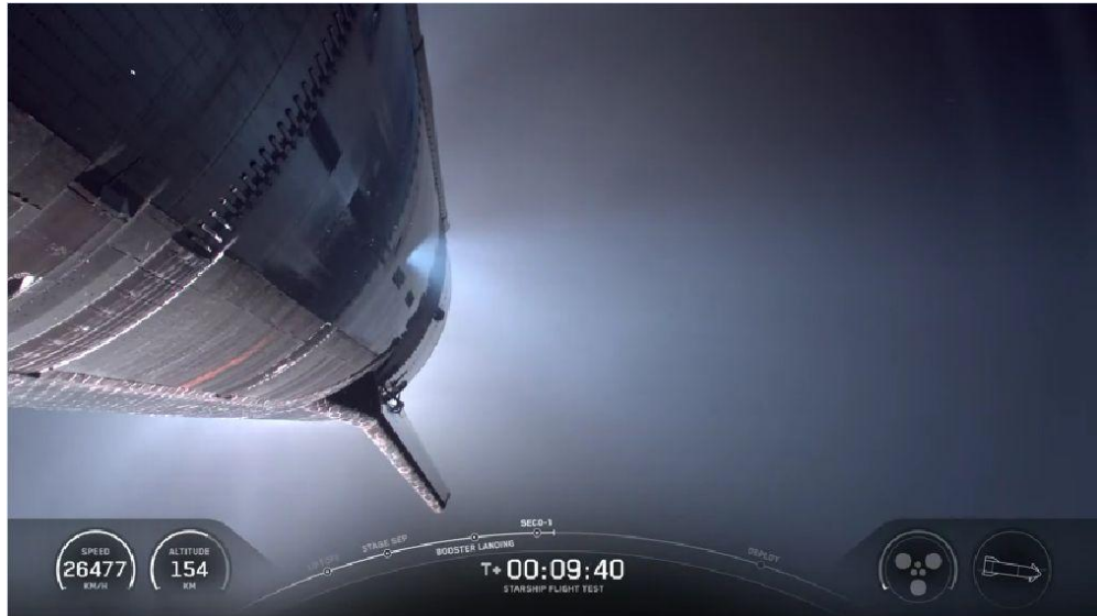
Fig. 10 – Gas leakage through the side wall of Starship second stage after its engines are cut off
