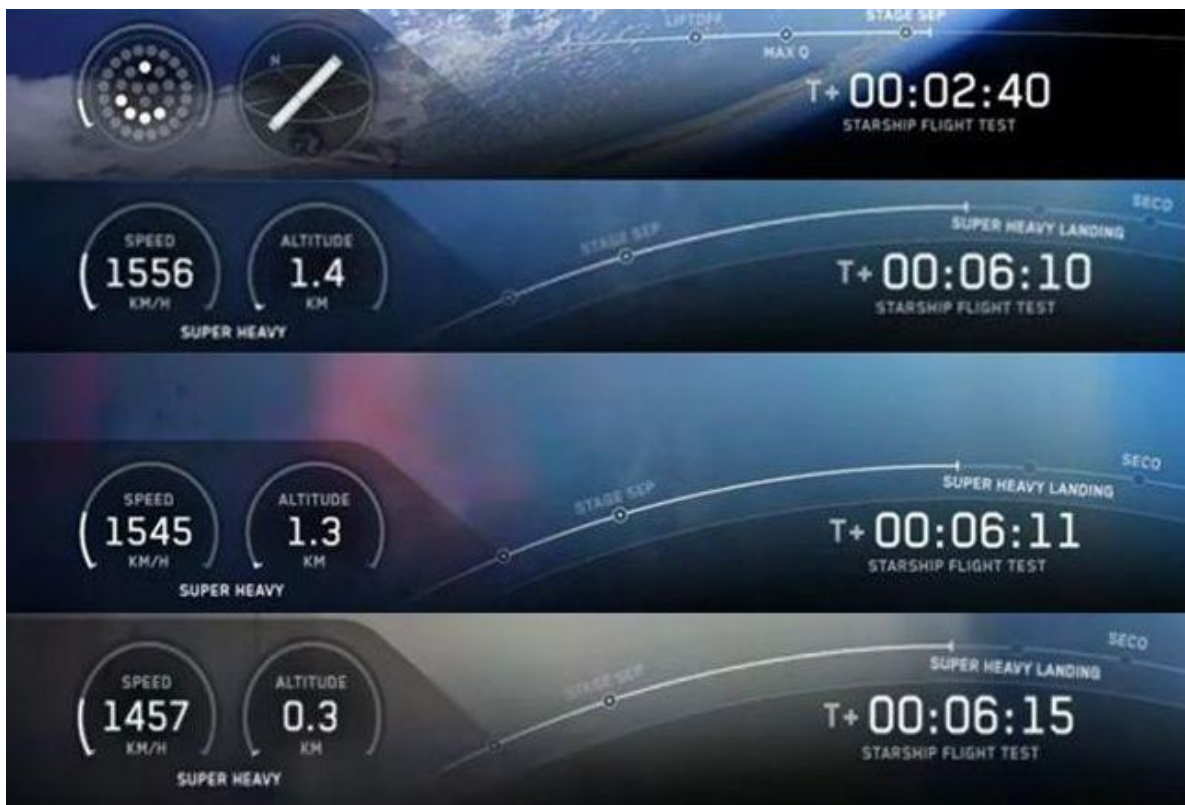
Fig. 2 – Trajectory and other telemetry data during the boostback burn and landing burn attempts of B19 booster [13]
