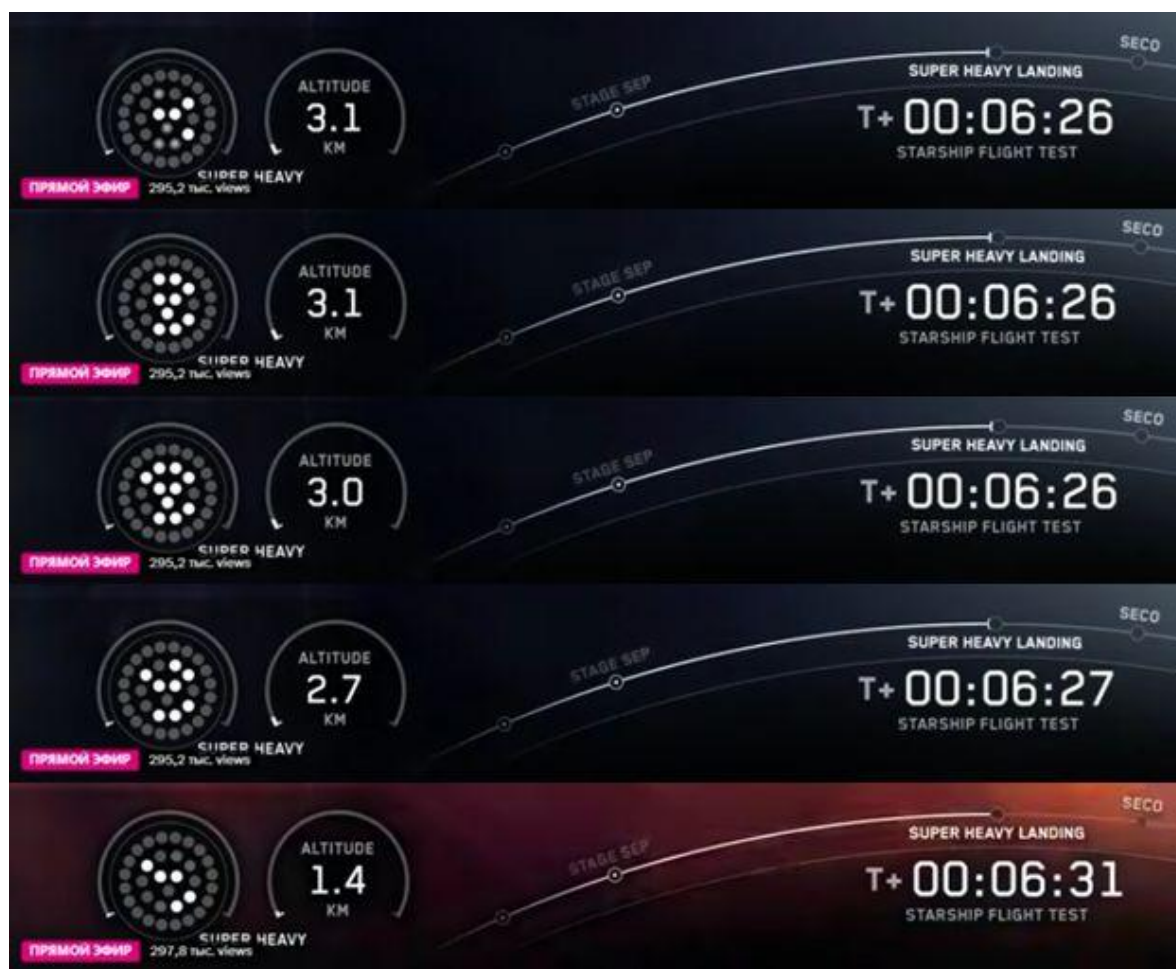
Fig. 5 – Activation and shutdown of B20 booster engines during its landing attempt [16]
