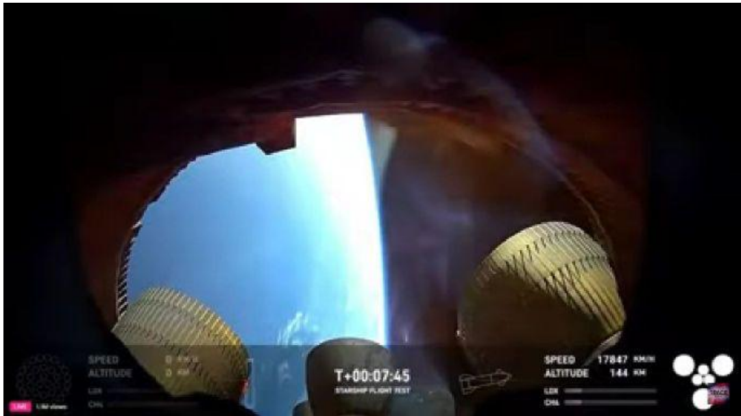
Fig. 8 – Reflection on the edge of the ship's attic a short flash of flame in its upper part during IFT-8
