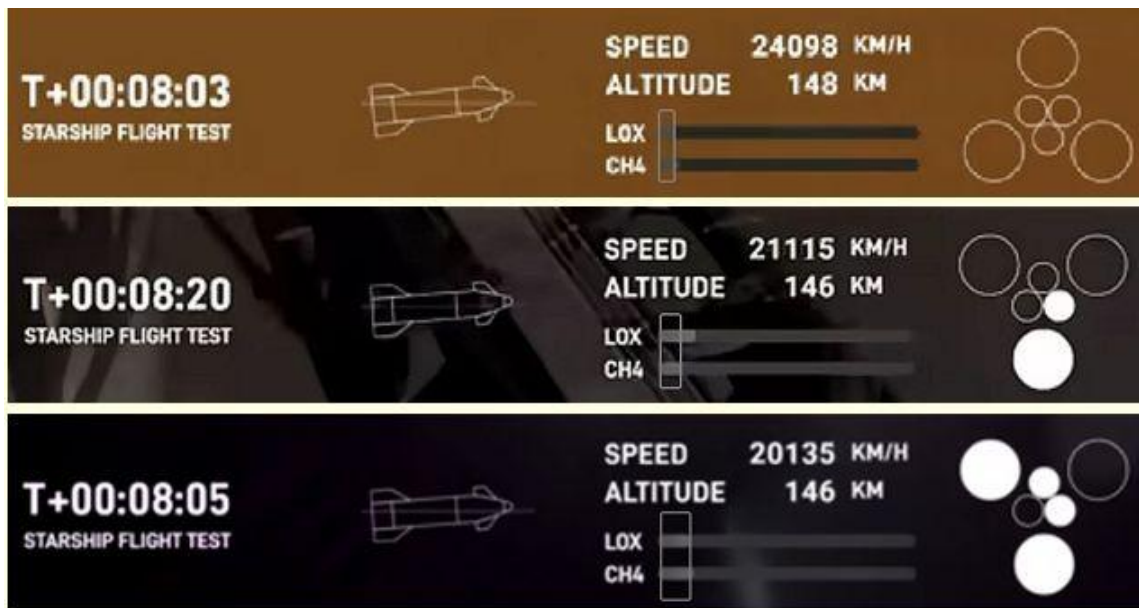
Fig. 10 – Oxygen and methane ratios in the tanks of Ships at IFT-2, IFT-7 and IFT-8 at the culmination moments of the three accidents
