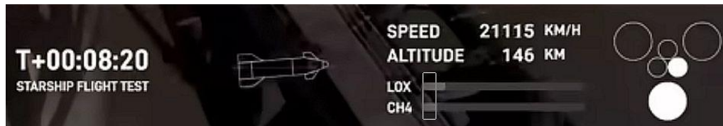
Fig. 7 – Ratio of oxygen and methane in the tanks of Ship during IFT-7 before the loss of telemetry
